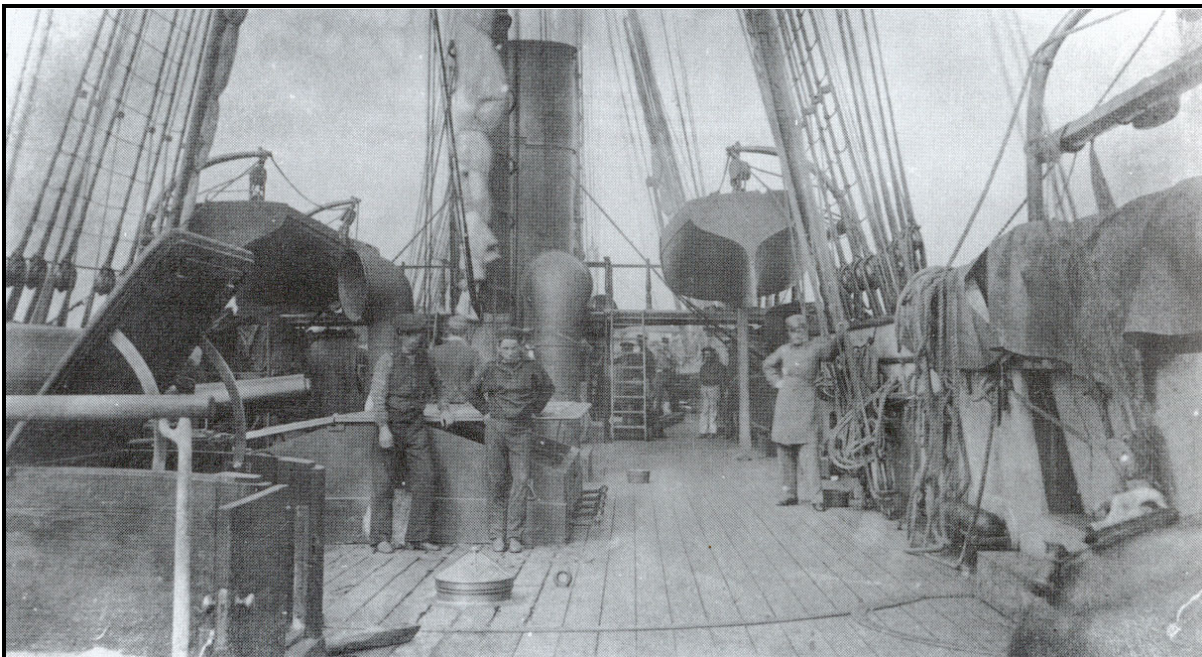
Figure 29. Breech of 100-pounder pivot rifle and muzzle of Fawcett Preston and Company 32-pounder beyond open companionway hatch.
